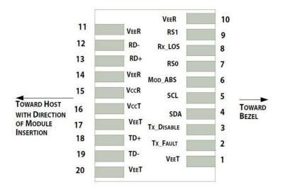
Pin-out of connector Block on Host board
