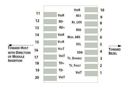
Pin-out of connector Block on Host board
