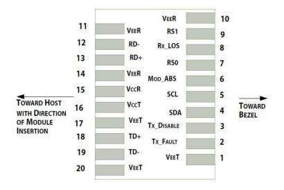
Pin-out of connector Block on Host board
