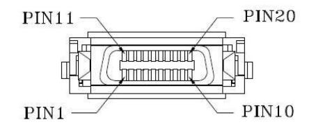
Pin-out of connector Block on Host board
