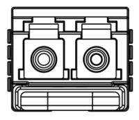
Looking into the connector, transmitter on the left.
